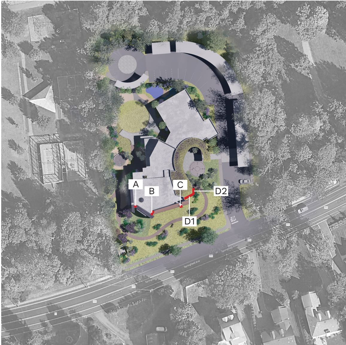
This image identifies all of the glazing areas that are fully visible from Springfield Avenue and were included in the glare study
